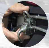
In the open position, the hook can be easily re-engaged and remains attached to the spreader bar
